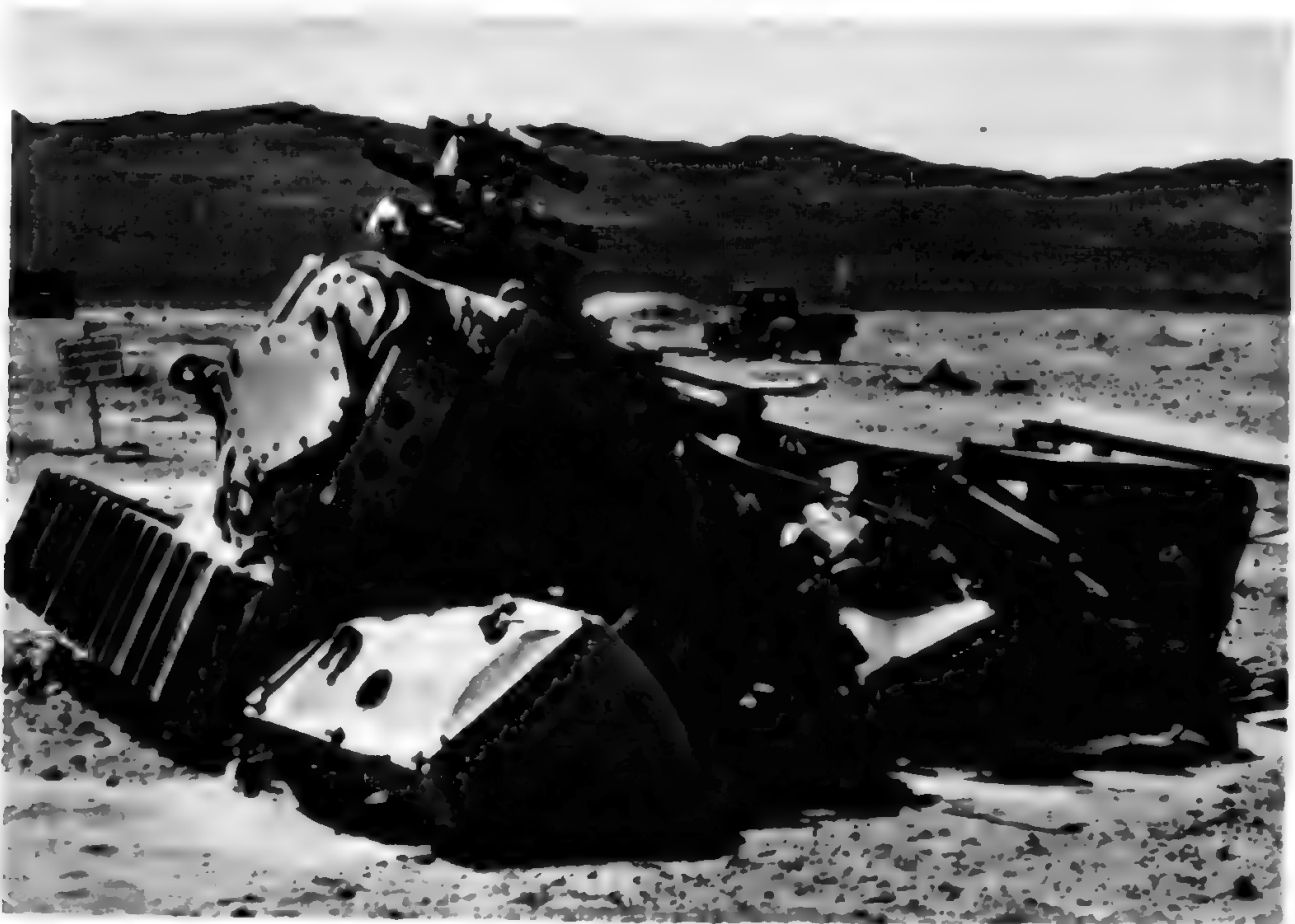
Figure 12.40b. Earth-moving equipment subjected to nuclear blast in open terrain (30 psi overpressure).
